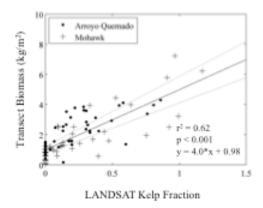
Figure 3. Validation of LANDSAT satellite biomass estimates. Linear regression analysis between LANDSAT kelp fractions and diver measured canopy biomass (kg/m²) measurements for Arroyo Quemado and Mohawk (n=96). The gray lines represent 95% confidence intervals for the relationship.
