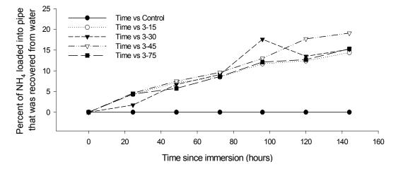
Figure 2. Dissolution rate of Ammonium from diffusers with 1 mm diameter holes at densities of 0-3.0 holes/cm of diffuser flexible PVC pipe. The legend refers to the third trial ("3") and the number of holes for each 25–cm long pipe (0-75).
